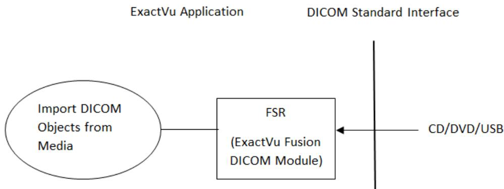
Figure 2: DICOM File-Set Reader Flow Diagram
